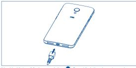
It is advised that you fully charge your battery ( ). Connect the battery charger to your phone and main socket respectively, charging status is indicated by the percentage on screen while the phone is powered off. The percentage increases as the phone is charged.
