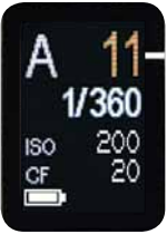
A glance at the OLED panel on the top deck of the Leica S shows its user the most important camera settings with commendable clarity. (Full-size view)
