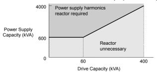
Figure i.3 Installing a Reactor
