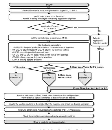
Figure 4.2 Basic Start-Up and Motor Tuning
