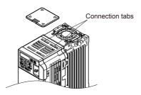
Figure 3.12 Reattaching the Top Cover
