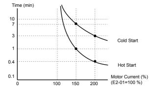
Figure 8.6 Motor Overload Protection Time
