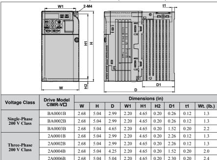
Table 2.3 IP20/Open-Chassis (without an EMC filter)
