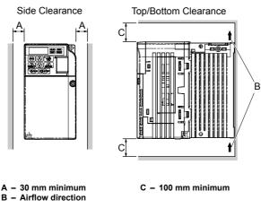
Figure 2.2 Correct Installation Spacing
