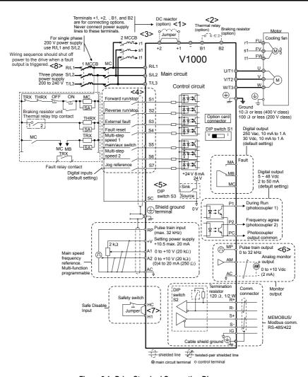
Figure 3.1 Drive Standard Connection Diagram
