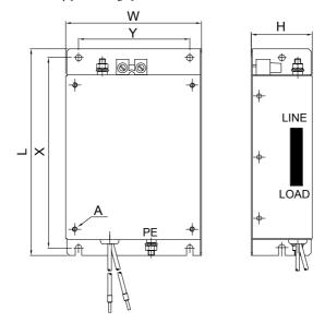
Figure 8.4 EMC Filter Dimensions
