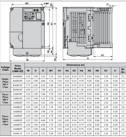
Table 2.6 IP20/NEMA Type 1 (without an EMC filter)
