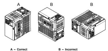
Figure 2.1 Correct Installation Orientation
