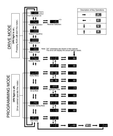
Figure 4.1 Digital LED Operator Screen Structure
