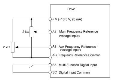
Figure 4.9 Switching between Main/Auxiliary Frequency References
