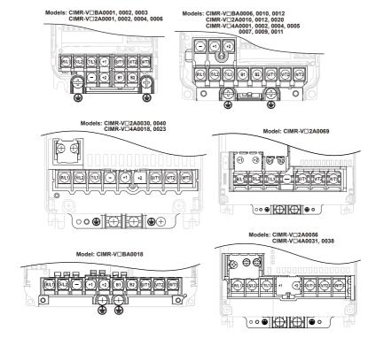
Figure 3.3 Main Circuit Terminal Block Configurations
