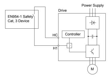
Figure 8.7 Safe Disable Wiring Example
