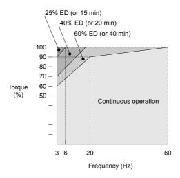
Figure i.4 Allowable Load Characteristics for a Yaskawa Motor
