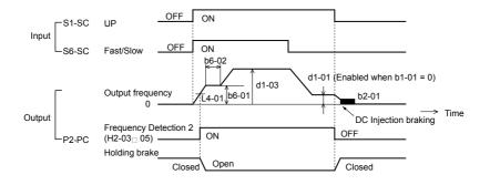
Figure 4.7 Holding Brake Time Chart
