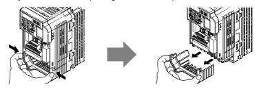
Figure 3.5 Remove the Terminal Cover on an IP20/Open-Chassis Drive
