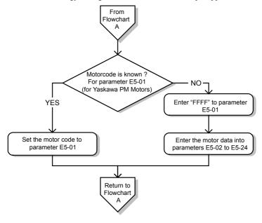
Figure 4.5 Operation with Permanent Magnet Motors
