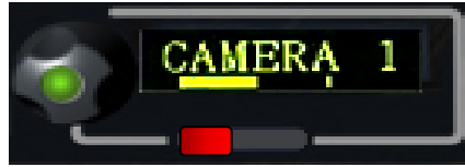
Figure 5-4: Rotary panel display: latched listen while talking
