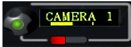
Figure 5-4: Rotary panel display: latched listen while talking
