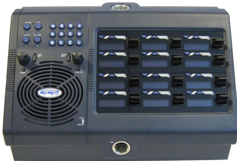
Figure 4-3: 'Upside down' desktop panel (for wall mounting)
