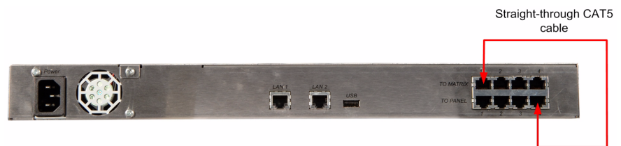
Figure 3-19: IP Reset Cable Setup
