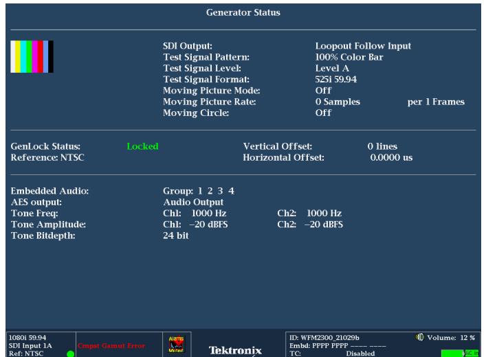
Generator Status display.
