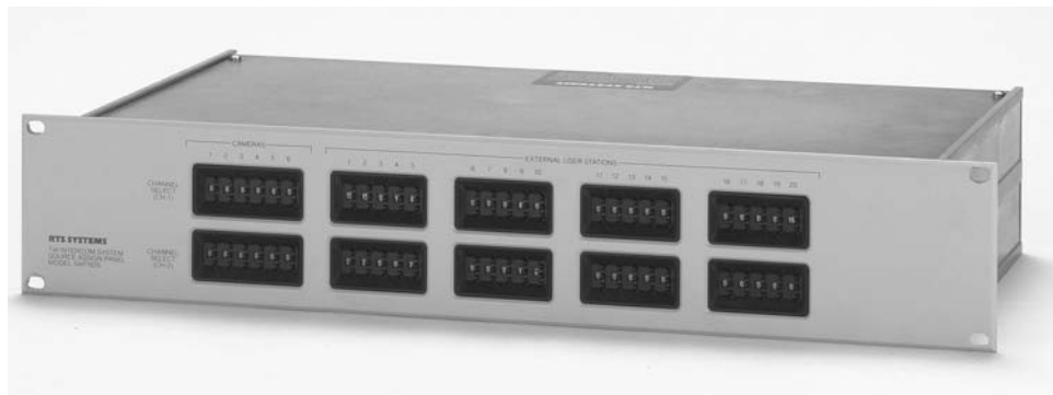
Figure 4.9 Use of Source Assignment Panels such as this SAP-1626 allow the rapid reconfiguration of PL systems without changing any cables
