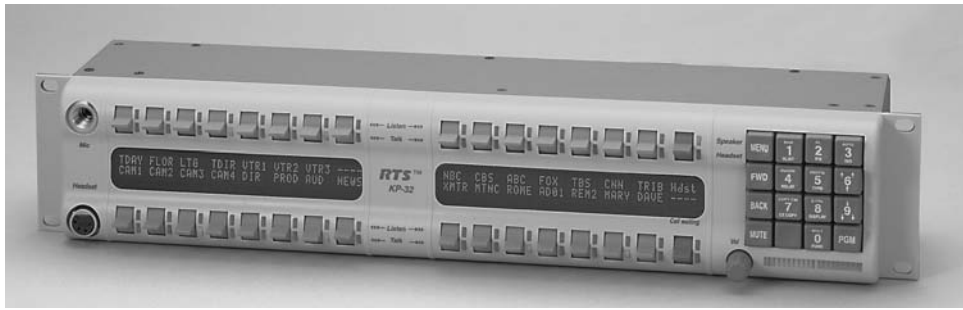
Figure 4.1 The KP-32 is a good example of an advanced user station (keypanel).
