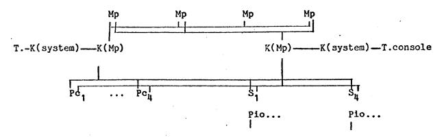
A failure anywhere can be tolerated. The K(Mp)'s have separate power. T.console communicates to all modules. Pc has a cache (write through) and each K(Mp) broadcasts writes to all Pc's on a physical memory basis. They're after reliability and incremented upgrade (since their customers buy and want more capability). They're also going after the performance title! The O/S modification was <u>very</u> hard, due to the structure of IBM's system.
