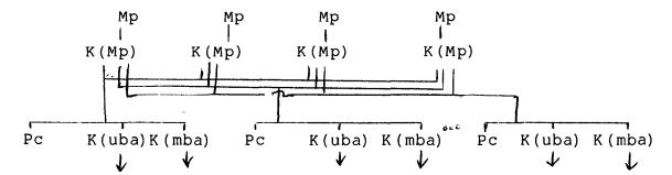
The place where the Fujitsu configuration may beat the DEC configuration is in intrinsic performance. As you describe it, Fujitsu does not have to explicitly turn off caching on pages that might potentially be shared between processors. DEC could use this strategy if we were willing to design the multiport memory controllers to broadcast all writes over the buses - though Fujitsu's scheme with several ports into all the Pc's looks like it will still give higher peformance.
