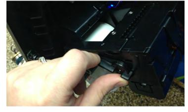
Turn the lever to open the print head, exposing the rollers.
