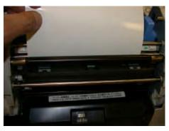
Insert between the metal and black rubber roller.
