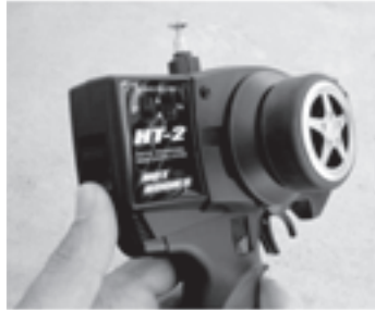
After the transmitter is on, turn on the receiver.
