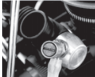
(A) Needle Valve Starting Position: Turn needle valve clockwise until it stops. (closed) Open counterclockwise 4 turns. (open)
