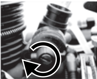
(C) If response on the lower rev is slow, turn the low speed needle valve clockwise (closed) by 30° increments until it shows better low rev response.
