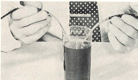
A foto-fade is made by dipping the end of the film into the dye for the distance the fade is to cover — then gradually withdrawing the film.
