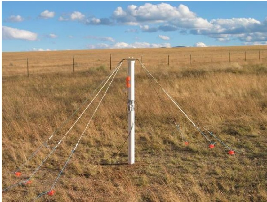
Figure 43: The fork antenna (without shorting braid across the bottom of each element). Photo obtained from [5].
