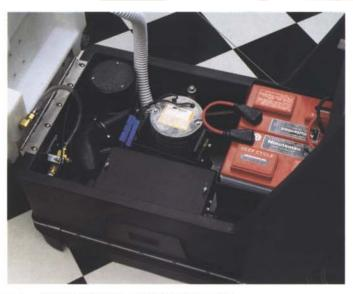
Simply raise the solution/recovery tank for easy access to deep cycle batteries and moisture protected components.
