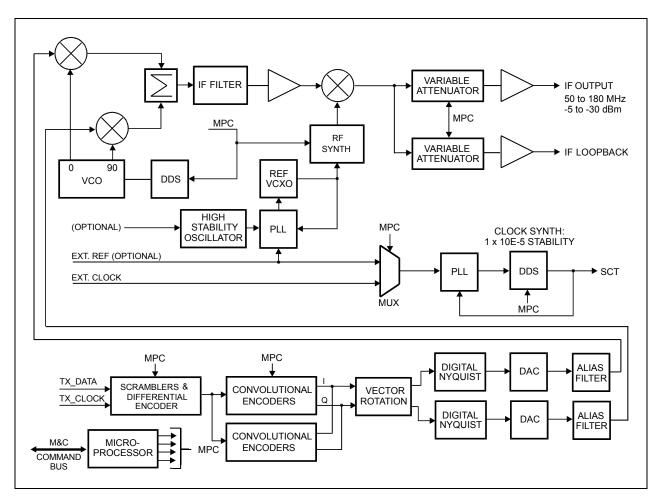
Figure 5-2. Modulator Block Diagram
