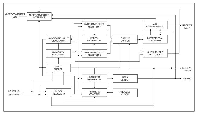
Figure B-1. Sequential Decoder Block Diagram
