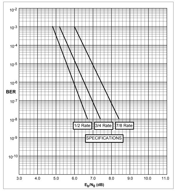
Figure C-3. Sequential Decoder, 1544 kbps BER Performance Curves
