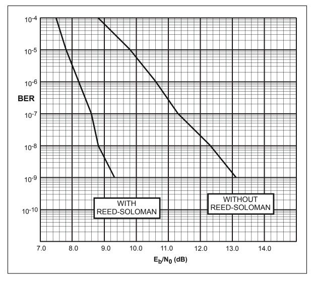
Figure C-6. Viterbi Decoder, 8-PSK 5/6 BER Performance Curves
