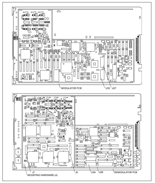
Figure B-2. Sequential Decoder Installation
