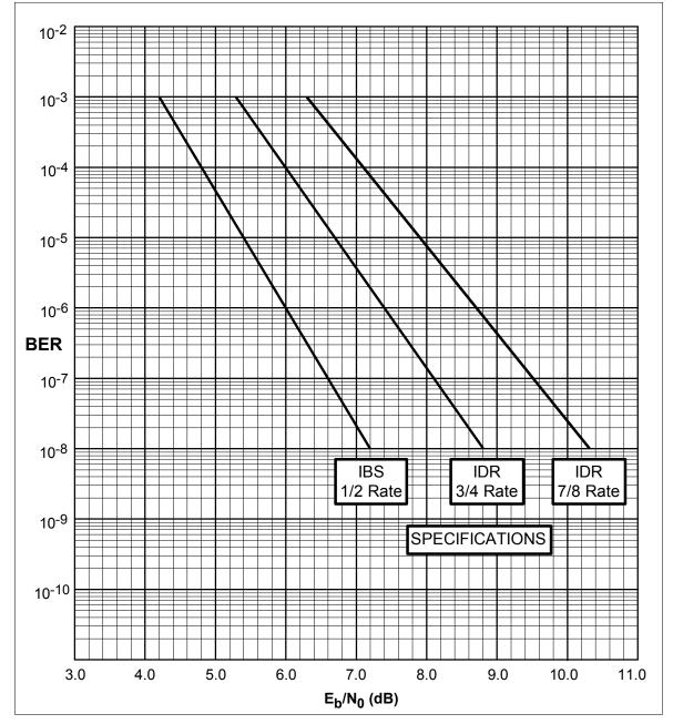
Figure C-1. Viterbi BER , IBS, and D&I Mode Performance Curves
