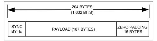
Figure B-17. 204-byte Mode Baseband Packet
