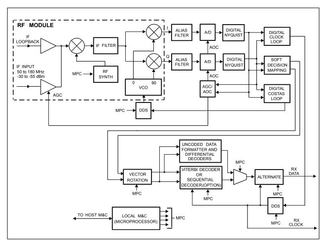
Figure 5-3. Demodulator Block Diagram
