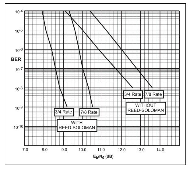
Figure C-7. Viterbi Decoder and 16-QAM
