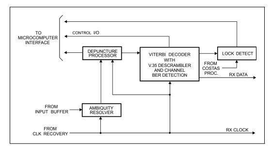
Figure 5-4. Viterbi Decoder Block Diagram
