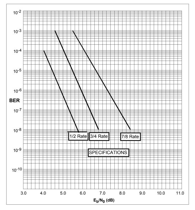
Figure C-2. Sequential Decoder 56 kbps BER Performance Curves
