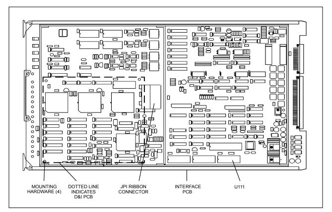
Figure B-4. D&I Multiplexer Installation
