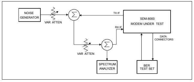
Figure 9-1. Fault Isolation Test Setup
