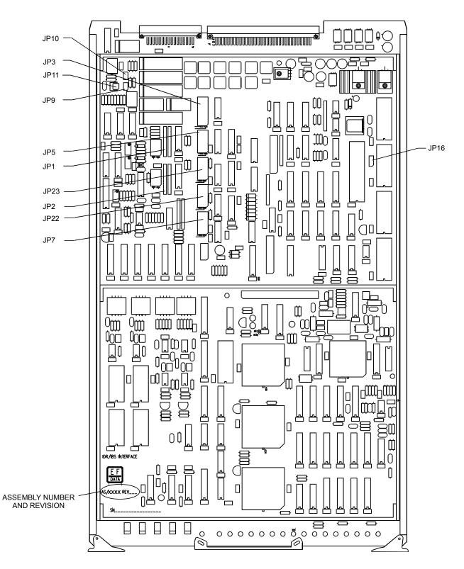
Figure 4-4. Interface PCB
