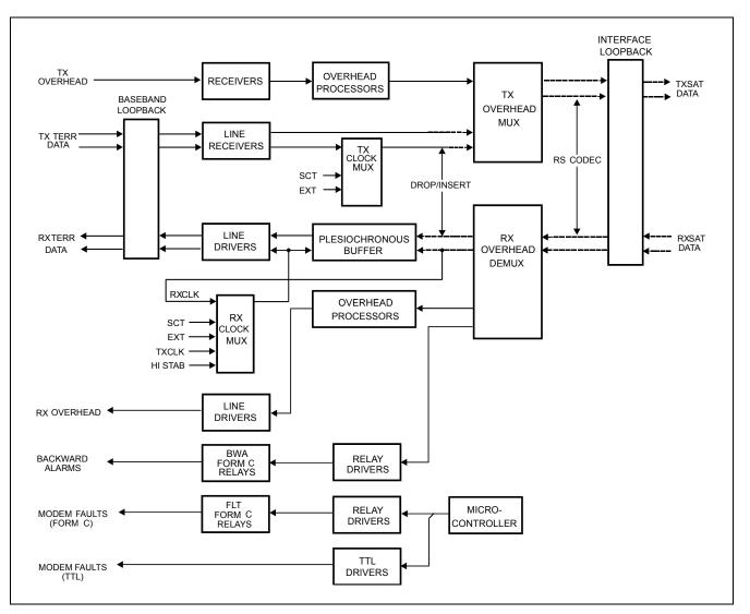
Figure 5-5. Interface Block Diagram
