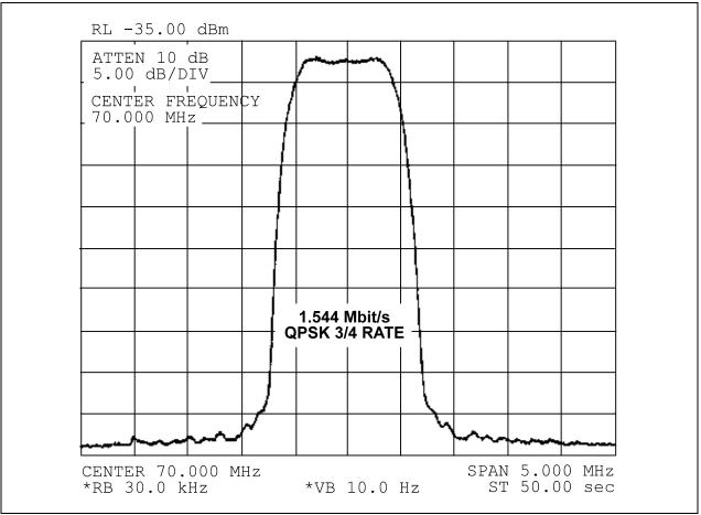
Figure C-8. SDM-8000 Typical Spectral Occupancy
