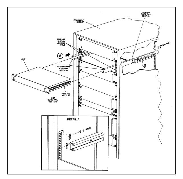
Figure 2-1. Typical Rack Installation
