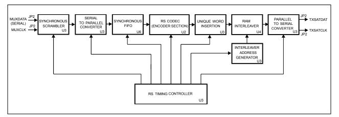
Figure B-6. Reed-Solomon Encoder Section Block Diagram
