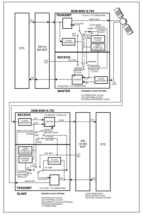
Figure 7-2. IDR/IBS G.703 Master/Slave Clocking Diagram
