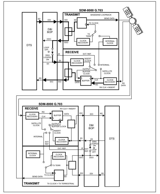
Figure 6-7. Baseband Loopback (with D&I)
