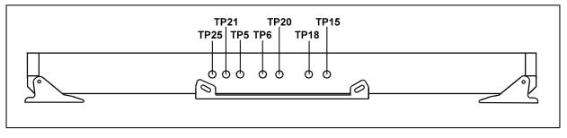
Figure 9-7. Demodulator PCB Test Points
