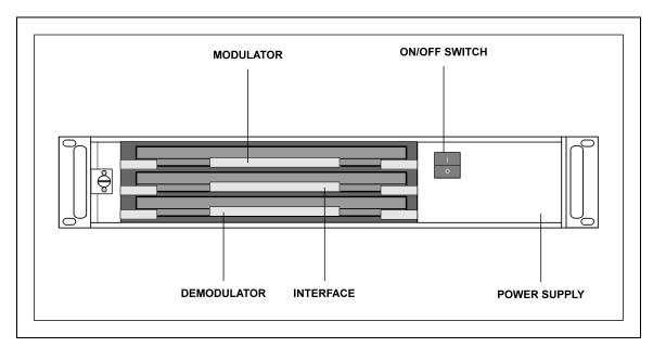
Figure 1-2. Modulator Construction
