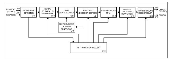
Figure B-8. Reed-Solomon Decoder Section Block Diagram
