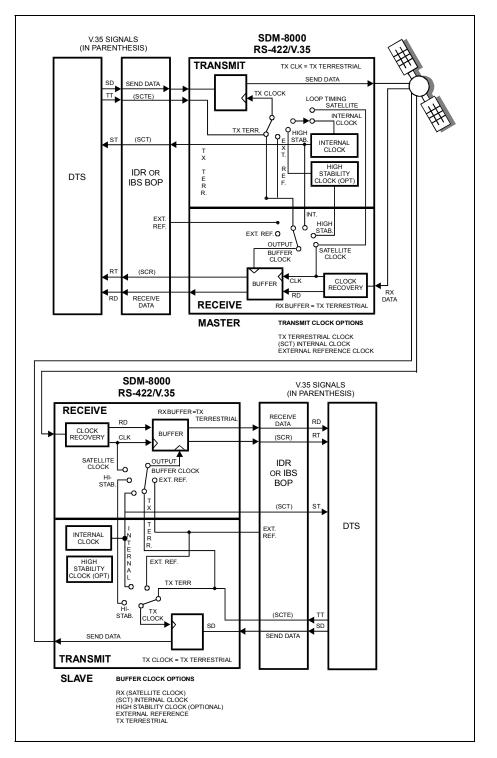
Figure 7-3. IDR/IBS EIA-422/V.35 Master/Master Clocking Diagram
