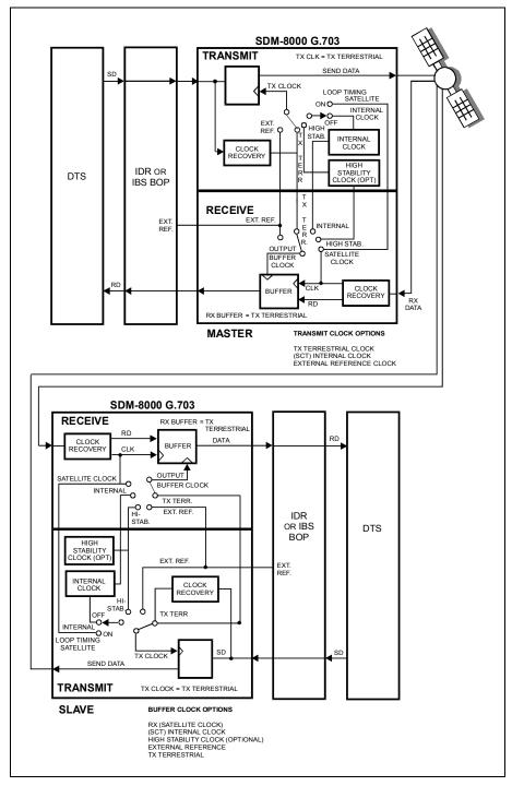
Figure 7-1. IDR/IBS G.703 Master/Master Clocking Diagram
