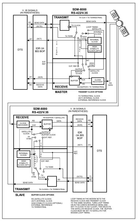
Figure 7-4. IDR/IBS EIA-422/V.35 Master/Slave Clocking Diagram
