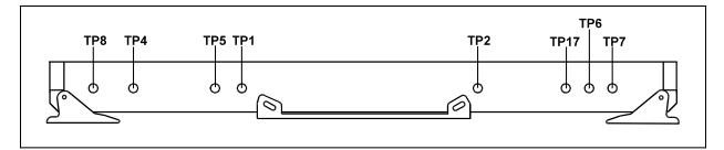
Figure 9-6. Modulator PCB Test Points
