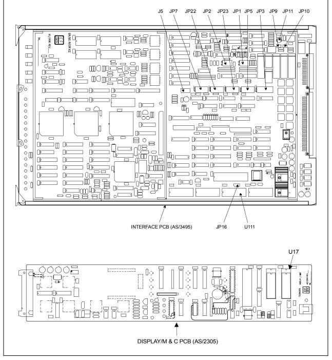
Figure B-11. Interface Relay Board Installation
