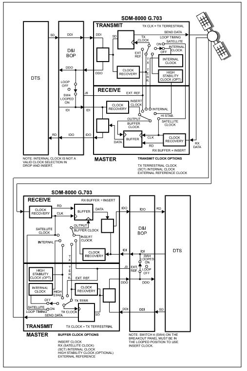
Figure 7-5. D&I G.703 Master/Master Clocking Diagram
