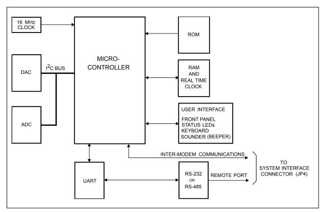
Figure 5-1. Display/M&C Block Diagram
