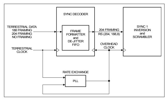
Figure B-14. Baseband Terrestrial Framing Block Diagram
