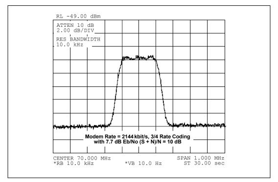
Figure 9-2. Typical Output Spectrum (with Noise)
