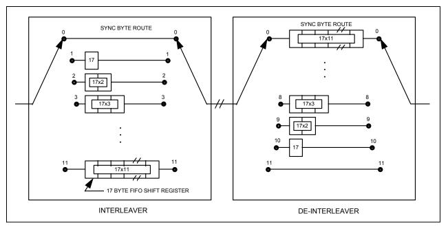
Figure B-21. Interleaver/De-interleaver
