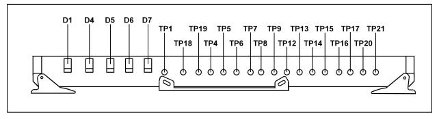
Figure 9-5. Interface PCB Test Points
