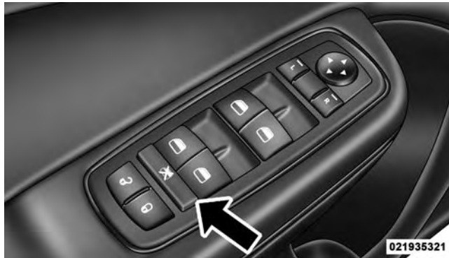
Window Lockout Switch
