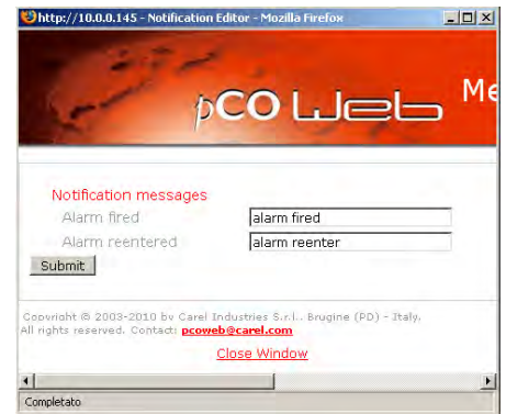
Figure 4.r – Setting the strings sent for Activation - Return
