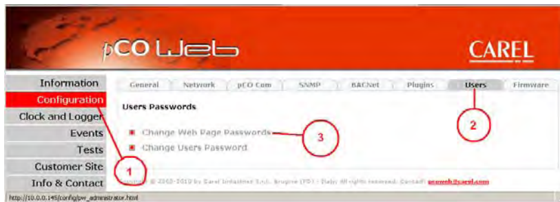
Figure 9.v – Protection and access control
