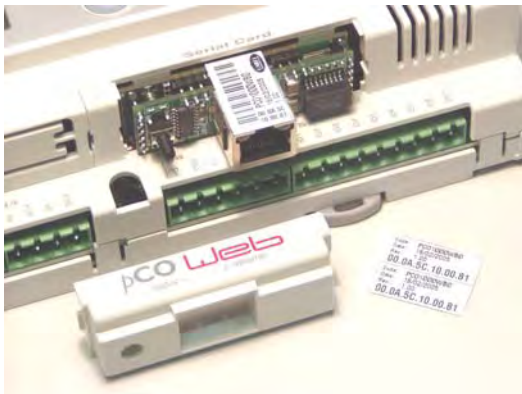
Figure 2.c – Inserting pCOWeb in the pCO controller
