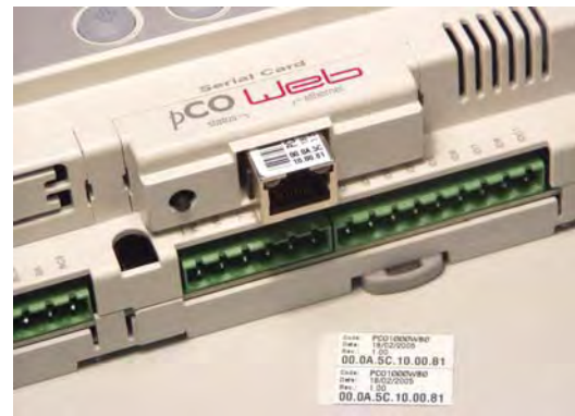
Figure 2.d – Securing pCOWeb with the cover
