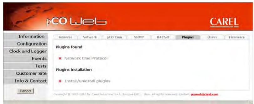
Figure 9.r – Plugin page after having installed “NTP”
