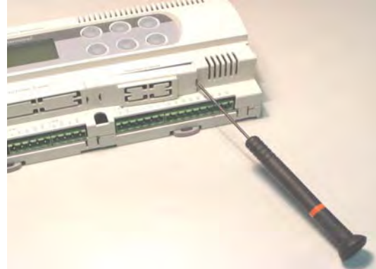
Figure 2.b – Removing the cover from the pCO controller
