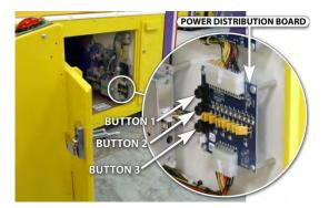
displayed on the LCD Display (located in the lower cabinet next to the main controller board), with the functions shown for Button 1 and Button 3.
