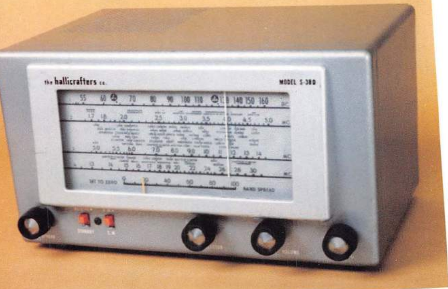
S-38D NONE 1955-57 $59.95 FIVE TUBES, SAME FREQUENCY COVERAGE, FEATURES AND SPECIFICATIONS AS THE S-38C BUT RADICALLY DIFFERENT APPEARANCE AS CAN BE SEEN. SLIDE RULE DIAL, SMOOTH LIGHT GRAY FINISH.
