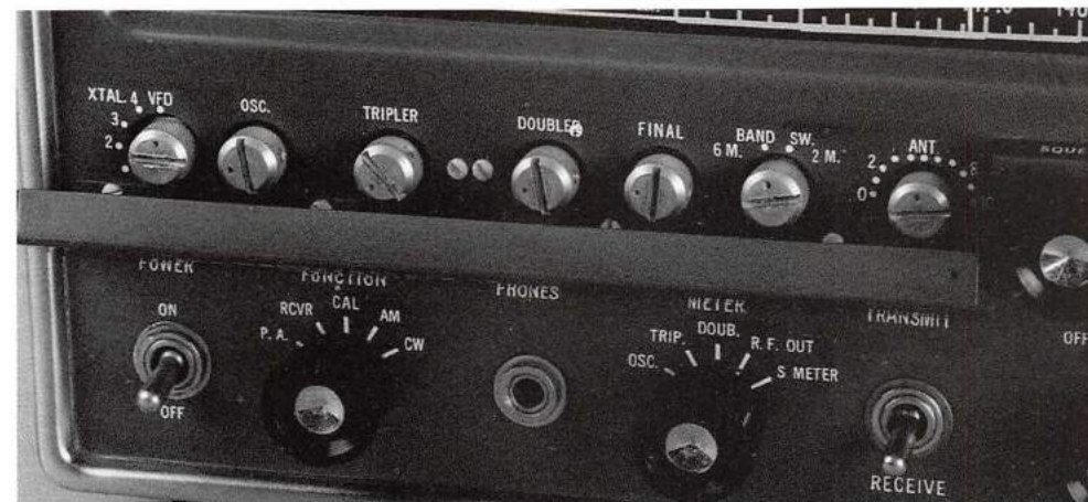
DETAIL OF CONTROLS HIDDEN BEHIND PANEL FLAP.
