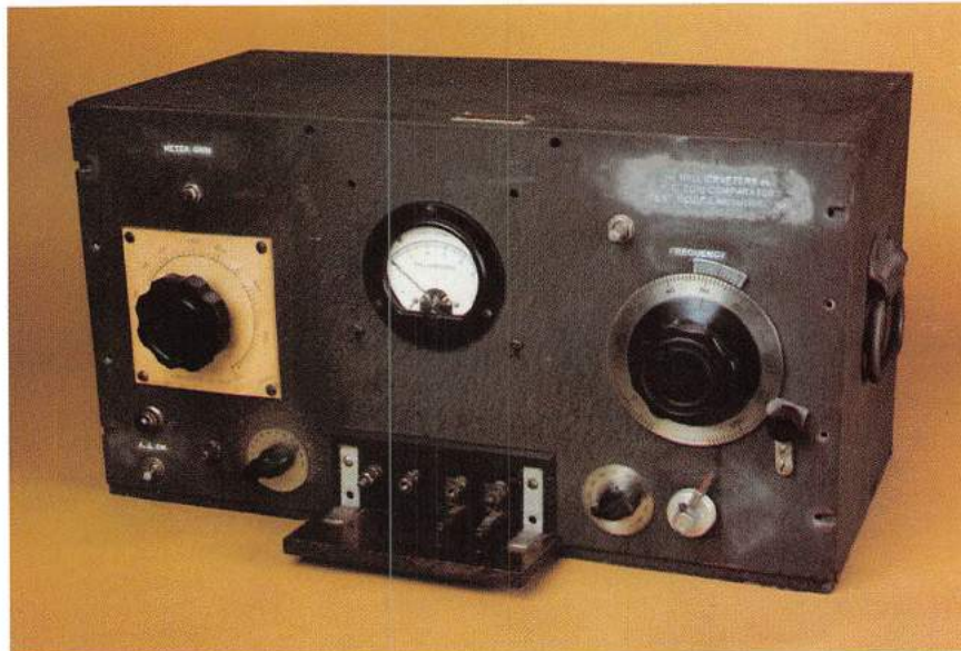
This one-of-a-kind unit is a model 101 R.F. Coil Comparator, a test unit built by the in-house test equipment laboratory. Its purpose was to check RF coils supplied by vendors to find "matched pairs" to be installed in the production equipment, circa 1940s. There wasn't time before the photo shoot to restore this unit, but that project is scheduled soon!
