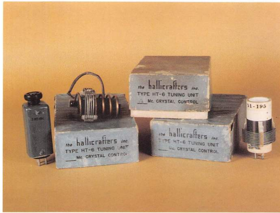
Tuning units and coils for the HT-6 with original boxes, circa 1939-45.
