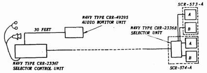
FIGURE 3.—Audio monitor unit, one selector control unit, one truck with two transmitters, and one truck with two receivers in block diagram relationship.
