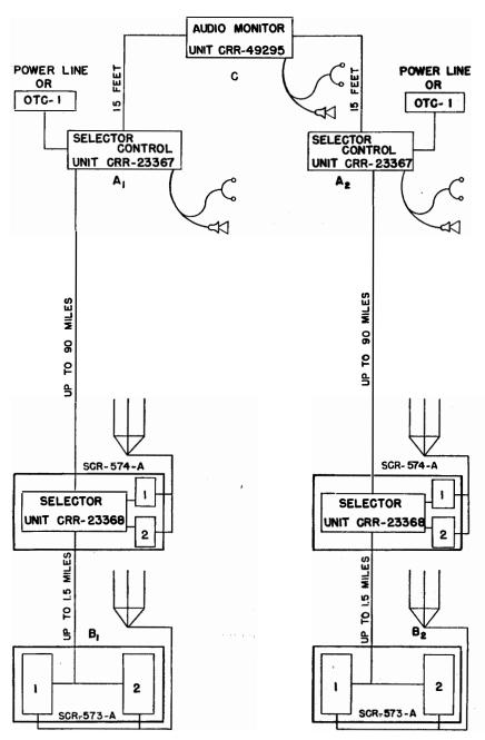
FIGURE 2.—Audio monitor unit, two selector control units, transmitting sets, and receiving sets in block diagram relationship.
