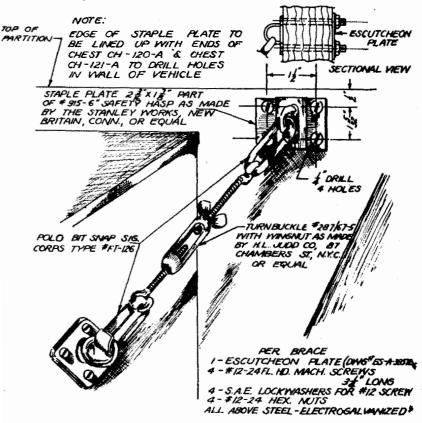
FIGURE 2.-Drawing of turnbuckle brace used to held chest in shelter.
