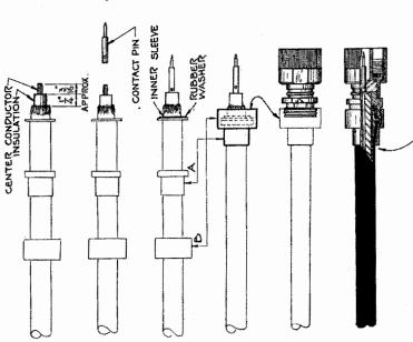
NOTE: IF CABLE IS ARMORED TERMINATE ARMOR ATAPPROX. THIS POINT & FASTEN WITH TAPE OR ANY OTHER SUITABLE MEANS.
