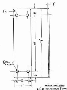
REINFORCING STRAP STEEL-BLACK CRACKLE FINISH 2 REQ. 2- STD. WASHERS FOR 1"BOLT 2- STD. S.A.E. LOCKWASHER FOR 1" BOLT
