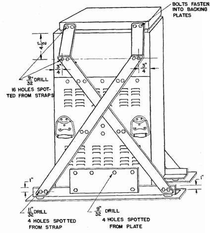
FIGURE 1.—Drawing of radio set SCR-399 with reinforcing modification.
