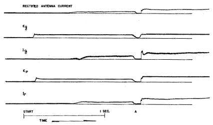
FIGURE 3.—Oscillographs showing conditions when equipment is started with test key closed and "adjust-tune-operate" switch in step No. 2. At time A it is switched to "operate."
