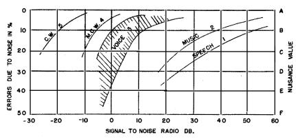
FIGURE 1.—Graph showing effect of signal to noise ratio on the intelligibility of signals.
