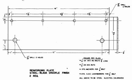
FIGURE 3.—Detail of reinforcing plate.
