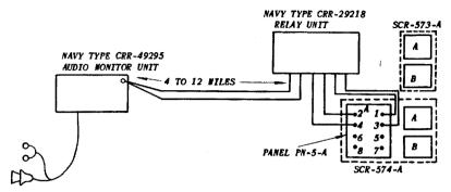
FIGURE 4.—Audio monitor unit, with relay unit, for controlling one truck with two transmitters and one truck with two receivers, in block diagram relationship,
