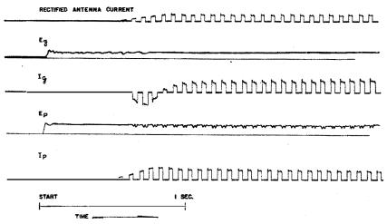
FIGURE 4.—Oscillographs with equipment operating on C. W. and keyed at 40 words per minute.
