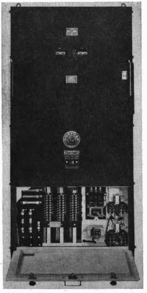
FIGURE 1.—Navy type CAY-20167, copper oxide rectifier power unit, front panel view.
