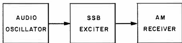
Figure 8-13.—Basic equipment setup for carrier balance adjustment.
