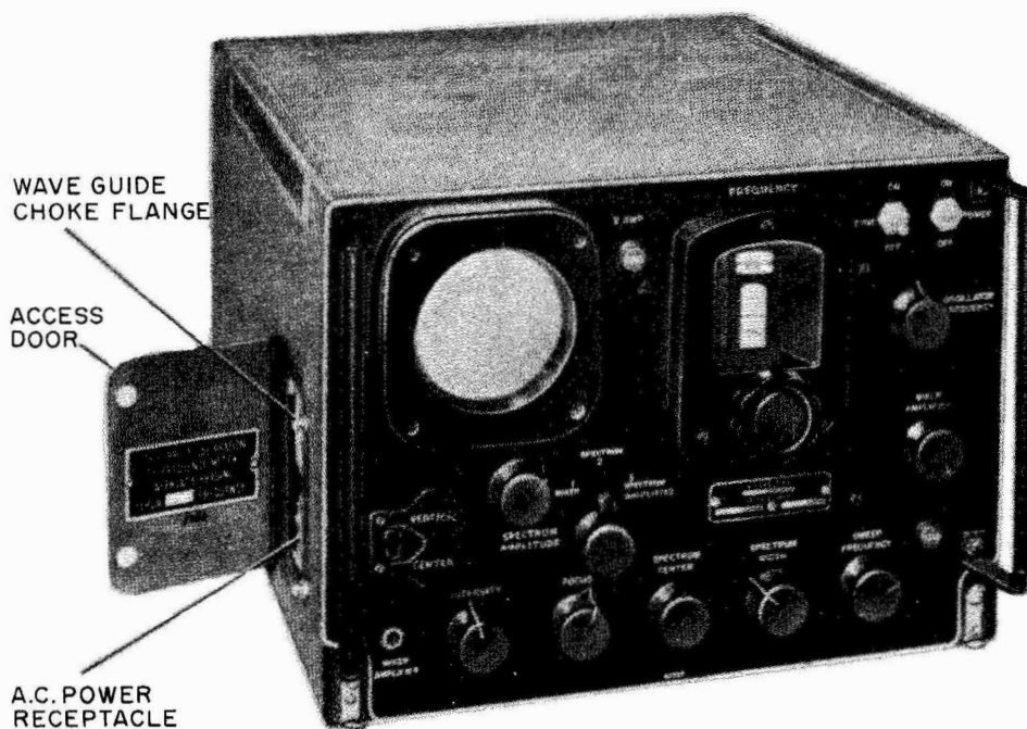
Figure 7-18.— Front-Panel of a typical spectrum analyzer.
