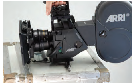
Finding the camera's fore-aft center of gravity.
