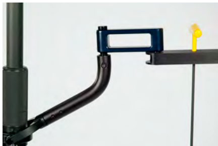
Balancing on the stand with the F-bracket attached.
