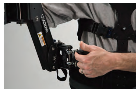
The arm socket is inserted into the socket block on the vest.
