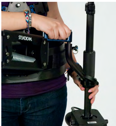
Hand positions for operating with the F-bracket.
