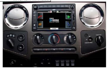
It can accept many of the same peripherals that a desktop PC uses such as keyboard, optical mouse, USB port, SD memory slot and much more. The computer as a standard has its basic new age functionality such as Bluetooth for phone connectivity and audio streaming from a music device. A special feature to the system is voice recognition & TTS which gives auditory feedback and commands. Safety is taken in consideration with the development of this computer.
