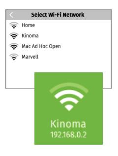
Clicking the "Select network" button displays a list of available networks. Select a network and enter password if necessary. Kinoma Create remembers the last configured Wi-Fi network.
