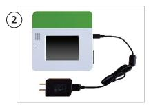
Begin charging device with supplied charger. (Note: Kinoma Create uses special charging circuitry and requires a sensing charger to correctly charge the battery. Only use the provided charger, since other chargers may not charge the battery).
