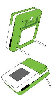
Kinoma create includes an adjustable stand. Use the dowels in the rear in the stand holes to set the stand to the angle desired.
