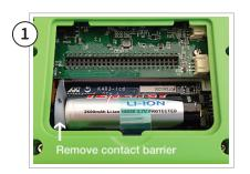
Remove back cover and pull out battery contact shield.
