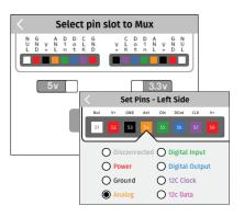
**Front Pins:** The 16 front facing pins can be targeted by the Front Pins app to support Digital, Analog In, and I2C connections. Power can be supplied at 3.3 or 5 volts. Input pins will handle up to 3.3v.
