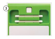
Press the power button on the back of Kinoma Create. Kinoma Create typically takes 35 seconds to boot up.
