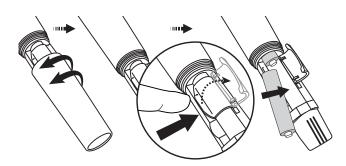
Unscrew the handheld Mic and open the battery cover to insert the battery into the battery compartment and confirm the marks of the polarity (+) (-).
