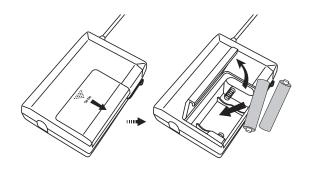
Open the battery cover and insert batteries into the battery compartment conforming to the polarity (+)(-) marks.
