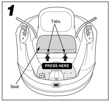
• If the seat has been assembled to your vehicle, press in on the tabs on the front of the seat and lift to remove it.
