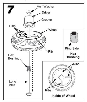
• Fit a hex bushing (ring side first), large wheel (inside surface up), driver (ring side first) and 7/16" (large diameter) washer on the long axle. Make sure that the grooves in the driver fit around the ribs on the rinside surface of the wheel.
