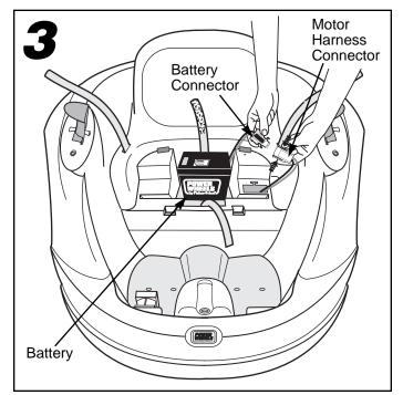
Squeeze the tabs on each side of the motor harness connector and plug the battery connector into the motor harness connector.
