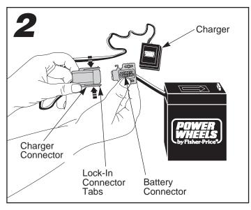
Squeeze the Lock-In connector tabs on the charger connector and plug it into the battery connector.
