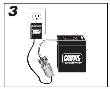
• Plug the charger into a standard 120 volt wall outlet.
