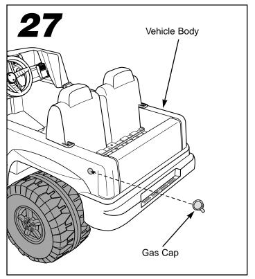
Fit the gas cap into the hole in the side of the vehicle body.
