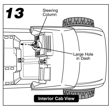
Fit the end of the steering column through the large hole in the dash.
