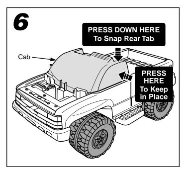
• Press firmly above one of the rear tabs to snap it into the slot in the vehicle body.
