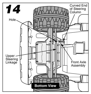
• From the underside of the vehicle body, fit the curved end of the steering column into the hole in the upper steering linkage.
