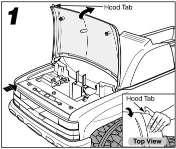
• Lift the hood to access the battery compartment. **Hint:** Place your hand on the vehicle body and "pop" the hood open by placing your hand under the hood tab (see inset).
