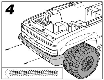
• Insert two #8-18 x 1<sup>3</sup>/<sub>4</sub>" screws through the holes in the front bumper and into the vehicle body. Tighten the screws using a Phillips screwdriver. Do not over-tighten.
