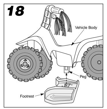
• Fit the footrest to the peg on the underside of the vehicle body .
