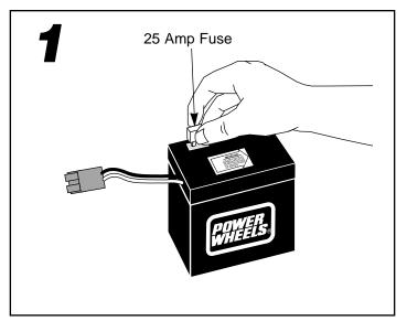
• Insert a 25 amp fuse into the battery.
