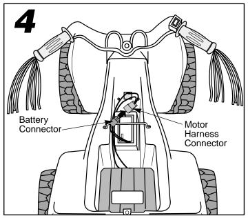
• Plug the battery connector into the motor harness connector. **Note:** If the battery connector will not plug into the motor
