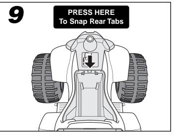
• Press firmly on the back of the cowling to snap the rear tab into the slots in the vehicle body.
