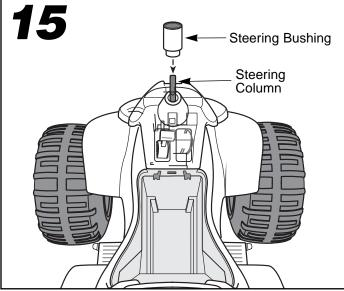
**Helpful Hint:** You may want the help of another adult to support the steering column near the steering linkage while assembling the handlebar to the vehicle body.
