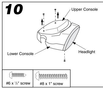
**Note:** For packaging reasons, the console/headlight has been pre-assembled at the factory. You will need to disassemble the console/headlight to assemble it to the handlebar.
