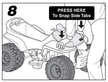
• Press firmly on each side of the cowling to snap the four side tabs into the slots in the vehicle body. Make sure the rear tab stays aligned with the slots.
