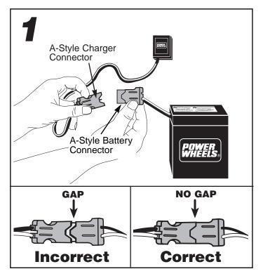
Plug the charger and battery connectors together. Push firmly to make sure the two connectors are completely joined.
