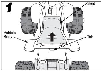
• Press the tab under the back of the seat and lift to remove the seat.
