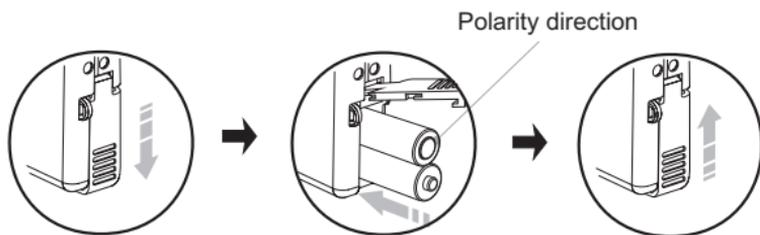
**Precaution:** Check the batteries for polarity. Remove the batteries if you are not going to use the camera. Do not short, disassemble or charge the batteries. Do not throw the batteries into a fire.
