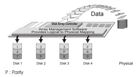
When RAID Level 5 technology is combined with cache memory to improve its write performance, the result can be used in any applications where general purpose disks would be suitable.
