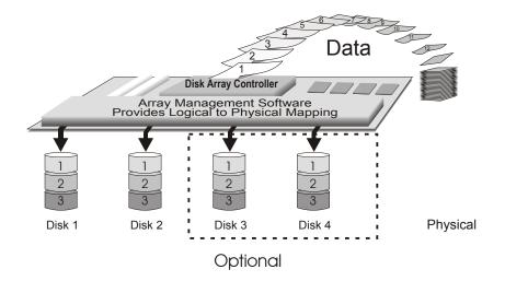
RAID level 1 provides both very high data reliability and continued data availability in the event of a failure of an array member. When a RAID level 1 member disk fails, array management software simply directs all application requests to the surviving member.
