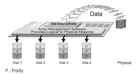
RAID Level 3 technology use a dedicated parity disk to store redundant information about the data on several data disks. RAID Level 3 is an excellent choice for applications which require single stream I/O with a high data transfer rate.
