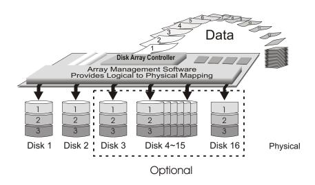
RAID level 1 provides both very high data reliability and continued data availability in the event of a failure of an array member. When a RAID level 1 member disk fails, array management software simply directs all application requests to the surviving member.
