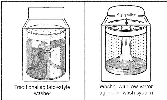
The most striking difference in your new washer is the low-water agi-peller wash system. The washer automatically adjusts the water level to the load size—no water level selector is needed.
