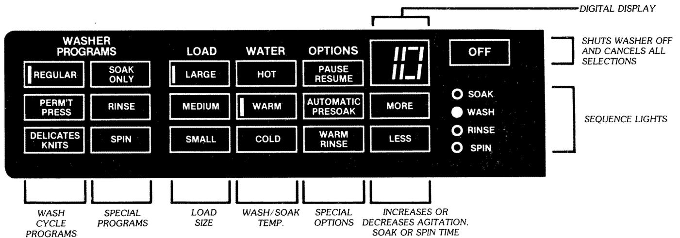
The left portion of the computer touch control panel programs the washer. The washer selections can be seen at a glance. Red indicators light up in the pads of the programmed selections.
