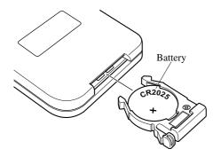
3. Press the battery case tab in the direction of the arrow until a click sound is heard.
