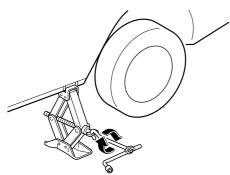
5. Remove the lug nuts by turning them counterclockwise; then remove the wheel and center cap.
