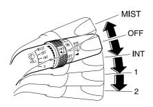
Turn the wipers on by pulling the lever down. MIST — Mist INT — Intermittent 1 — Low speed 2 — High speed
