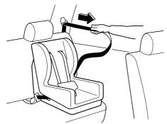
5. Push the child-restraint system firmly into the vehicle seat. Be sure the belt retracts as snugly as possible. Clicking from the retractor will be heard during retraction if the system is in the automatic locking mode. If the belt does not lock the seat down tight, repeat this step.
