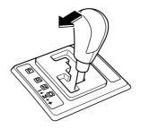
To return to automatic shift mode, shift the lever from M to D.
