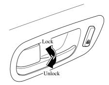
To lock any door with the door-lock knob from the outside, push the door-lock knob to the lock position and close the door. This does not operate the other door locks.
