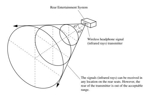
A wireless headphone can be used in any position on the rear seats, however, the sound may skip under the following conditions because the acceptable range varies or the signals are blocked.
