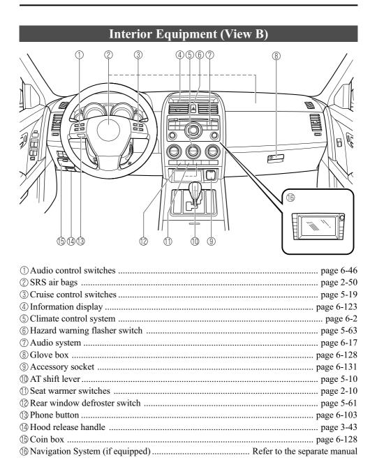
The equipment and installation position varies by vehicle **1-3**
