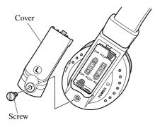
2. Insert two AAA-size batteries. Match the+ polarity of the batteries with the+ and- marks in the battery case.
