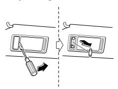
3. Install the new bulb in the reverse order of removal.
