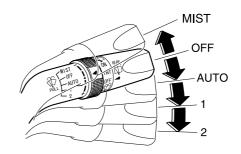
Turn the wipers on by pulling the lever down. MIST — Mist AUTO — Auto control 1 — Low speed 2 — High speed
