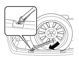
12. Pull the belt end to secure the flat tire.
