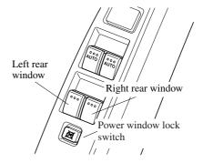
To open the power window to the desired position, hold down the switch. To close the power window to the desired position, pull up the switch.
