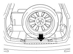
11. Thread the belt through the wheel as shown in the figure, then attach the belt clips to the hook.
