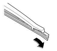
4. Remove the metal stiffeners from each blade rubber and install them in the new blade.
