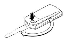
To retract the key, rotate it into the holder while pressing the release button.
