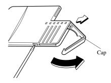
Do not turn the cap excessively. The cap may be damaged.
