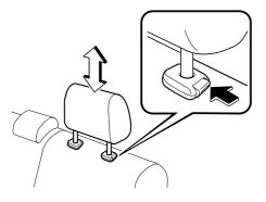
Adjust the head restraint so that the top is even with the top of the passenger's ears, never the passenger's neck to prevent injury.
