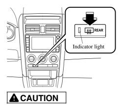
Don't use sharp instruments or window cleaners with abrasives to clean the inside of the rear window surface. They may damage the defroster grid inside the window. CX-9\_8V83-EA-06I\_Edition3 Page224 Monday, February 26 2007 7:19 PM
