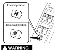
Unless a passenger needs to operate a power window, keep the power window lock switch in the locked position:
