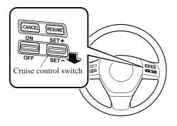
Your vehicle has a tap-down feature that allows you to decrease your current speed in decrements of 1.6 km/h (1 mph) by a momentary tap of the cruise control switch. Multiple taps will decrease your vehicle speed 1.6 km/h (1 mph) for each tap.
