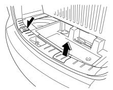
7. Remove the belt for securing the flat tire.
