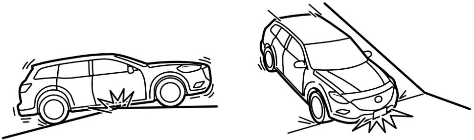
Your vehicle is equipped with low profile tires allowing class-leading performance and handling. As a result, the sidewall of the tires are very thin and the tires and wheels can be damaged if driven through potholes or on rough/uneven roads at excessive speeds. Use care and reduce speed when traveling on rough/uneven roads or through potholes.
