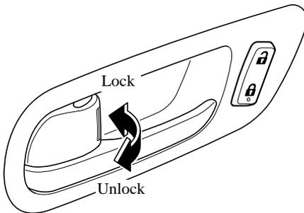
To lock any door with the door-lock knob from the outside, press the door-lock knob to the lock position and close the door. This does not operate the other door locks.
