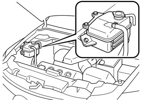
If it is at or near L, add enough coolant to the coolant reservoir to provide freezing and corrosion protection and to bring the level to F.
