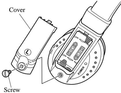
2. Insert two AAA-size batteries. Match the + polarity of the batteries with the + and - marks in the battery case.
