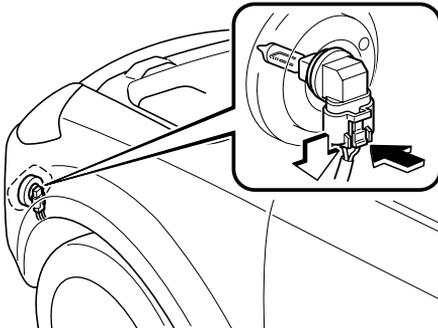
5. Turn the socket and bulb assembly counterclockwise and remove it. Carefully remove the bulb from its socket in the reflector by gently pulling it straight backward out of the socket.
