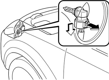
6. Turn the socket and bulb assembly to remove it. Carefully remove the bulb from its socket in the reflector by gently pulling it straight backward out of the socket.
