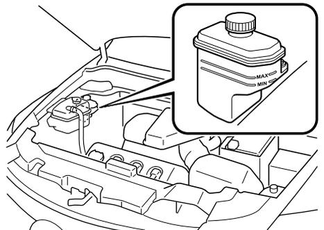
The level must be kept between MAX and MIN.
