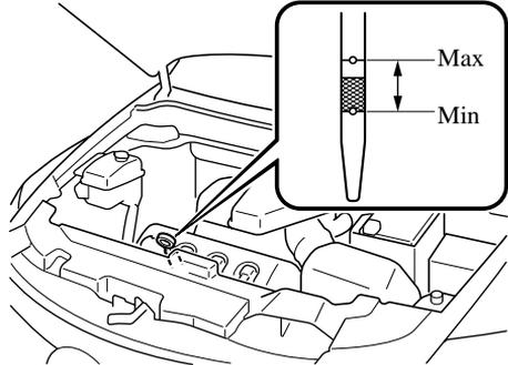
5. Pull it out again and examine the level. The level is normal if it is between MIN and MAX. If it is below MIN, add oil to raise the level within the hatching zone.
