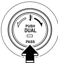
Use the DUAL switch to change the mode between the individual operation (driver and passenger) and interconnection (simultaneous) modes.
