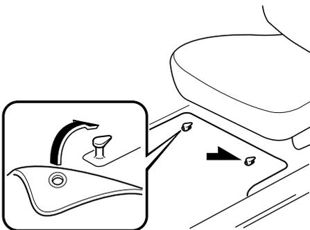
When setting a floor mat, position the floor mat so that its eyelets are inserted over the pointed end of the retention posts.
