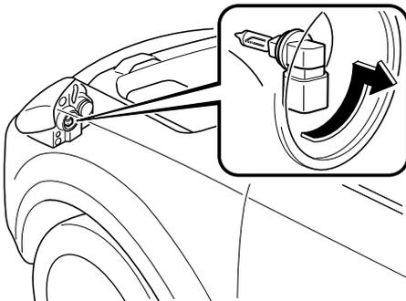
7. Install the new bulb in the reverse order of the removal procedure.
