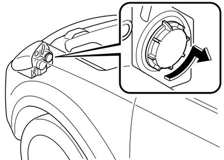
4. Turn the socket and bulb assembly counterclockwise and remove it.
