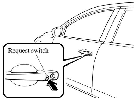
To stop the windows and the moonroof from closing, release the request switch. If the operation is performed from the beginning again, the windows and the moonroof close.
