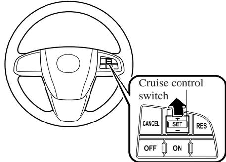
Your vehicle has a tap-up feature that allows you to increase your current speed in increments of 1.6 km/h (1 mph) by a momentary tap of the cruise control SET + switch. Multiple taps will increase your vehicle speed 1.6 km/h (1 mph) for each tap.
