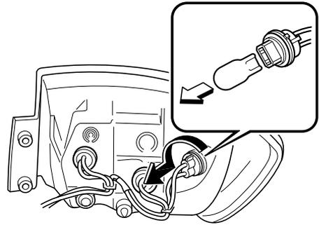
5. Disconnect the bulb from the socket.
