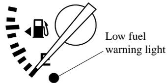
This warning light in the fuel gauge signals that the fuel tank will soon be empty. Refuel as soon as possible.
