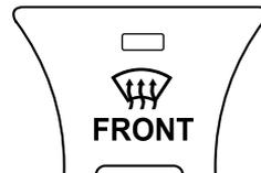
Press the switch to defrost the windshield and front door windows.
