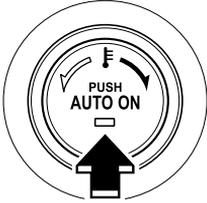
2. Use the temperature control dial to select a desired temperature. Press the DUAL switch or turn the front passenger temperature control dial to control the set temperature individually for the driver and front passenger.
