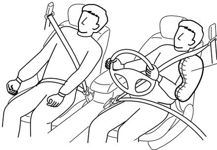
A side air bag will deploy only on the side the vehicle receives the force of the impact.
