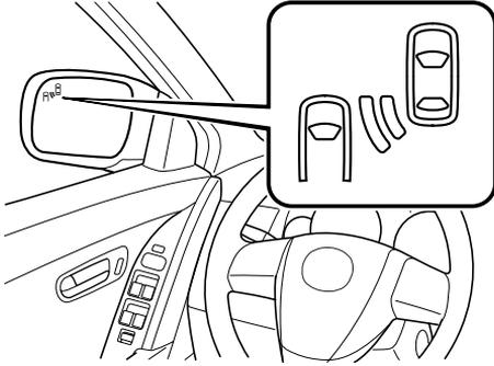
This warning light illuminates for a few seconds when the ignition is switched ON.
