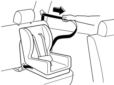
7. Push the child-restraint system firmly into the vehicle seat. Be sure the belt retracts as snugly as possible. A clicking noise from the retractor will be heard during retraction if the system is in the automatic locking mode. If the belt does not lock the seat down tight, repeat this step.
