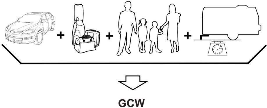
**GCW (Gross Combination Weight)** is the weight of the loaded vehicle (GVW) plus the weight of the fully loaded trailer.
