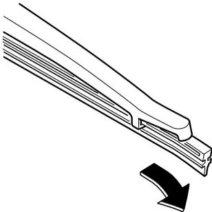
4. Remove the metal stiffeners from each blade rubber and install them in the new blade.
