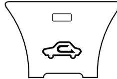
Outside or recirculated air positions can be selected. Press the switch to select outside/recirculated air positions.
