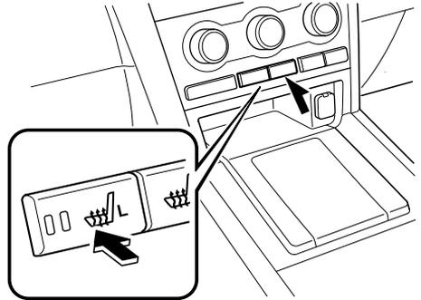
Press the seat warmer switch to illuminate the indicator light while the ignition is switched ON. The mode changes as follow each time the seat warmer switch is pressed.
