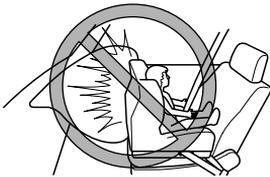
**Do not use a rearward facing child restraint on a seat protected by an airbag in front of it.**
