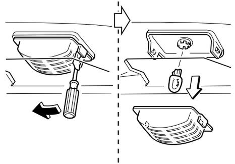
4. Install the new bulb in the reverse order of the removal procedure.
