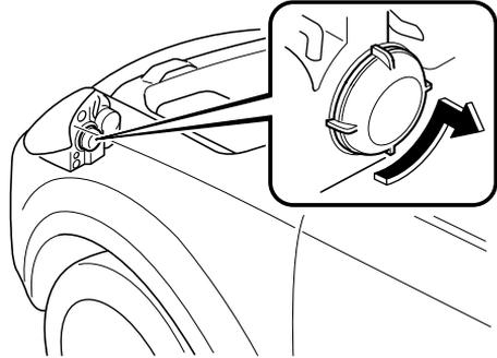
5. Disconnect the electrical connector from the bulb by pulling the tab on the connector with your finger and pulling the connector downward.
