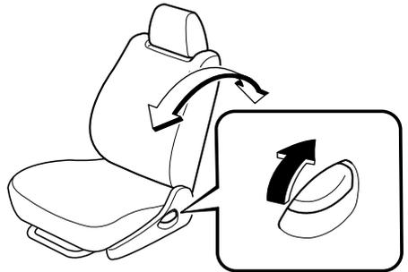
Make sure the lever returns to its original position and the seatback is locked in place by attempting to push it forward and backward.
