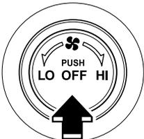
Pressing the OFF switch shuts off the climate control system.
