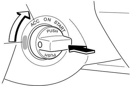
9. Switch the ignition from ACC to START and hold (up to 10 seconds at a time) until the engine starts.
