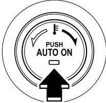
By pressing the AUTO switch the following functions will be automatically controlled in accordance with the selected set temperature:
