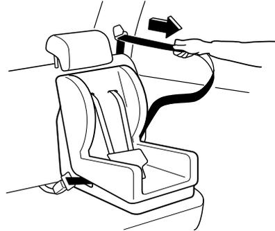
4. Push the child-restraint system firmly into the vehicle seat. Be sure the belt retracts as snugly as possible. Clicking from the retractor will be heard during retraction if the system is in the automatic locking mode. If the belt does not lock the seat down tight, repeat this step.
