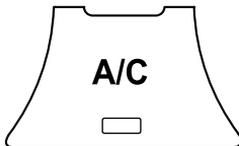
Pressing the A/C switch while the AUTO switch is turned on will turn off the air conditioning (cooling/dehumidifying functions). The air conditioning can be turned on and off by pressing the A/C switch while the fan control dial is on.
