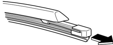
6. Remove the metal stiffeners from each blade rubber and install them in the new blade.
