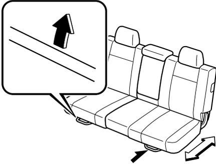
Make sure the bar returns to its original position and the seat is locked in place by attempting to push it forward and backward.
