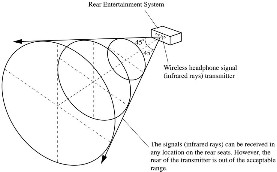
A wireless headphone can be used in any position on the rear seats, however, the sound may skip under the following conditions because the acceptable range varies or the signals are blocked.
