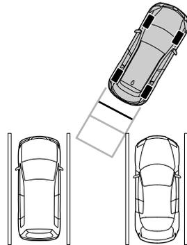
3. After your vehicle begins entering the parking space, continue backing up slowly so that the distance between the vehicle width lines and the sides of the parking space on the left and right are roughly equal.
