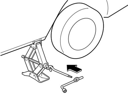
7. Turn the lug wrench clockwise and raise the vehicle high enough so that the spare tire can be installed. Before removing the lug nuts, make sure your Mazda is firmly in position and that it cannot slip or move.
