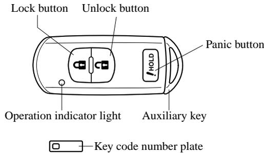
A code number is stamped on the plate attached to the key set; detach this plate and store it in a safe place (not in the vehicle) for use if you need to make a replacement key.
