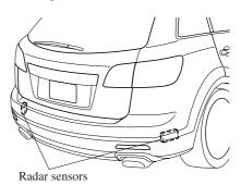
Always keep the bumper surface near the radar sensor area clean so that the BSM system operates normally. Refer to the Exterior Care (page 8-56).
