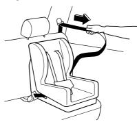
4. Push the child-restraint system firmly into the vehicle seat. Be sure the belt retracts as snugly as possible. Clicking from the retractor will be heard during retraction if the system is in the automatic locking mode. If the belt does not lock the seat down tight, repeat this step.
