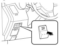
Press the switch again to turn the TCS back on. The TCS OFF indicator light will turn off. If the vehicle speed is more than 15 km/h (9 mph), the TCS OFF indicator light will not illuminate even if the switch is pressed.
