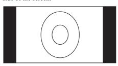
\* A 16:9 screen ratio image is scaled to a 4:3 screen ratio.
