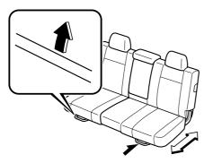
Make sure the bar returns to its original position and the seat is locked in place by attempting to push it forward and backward.
