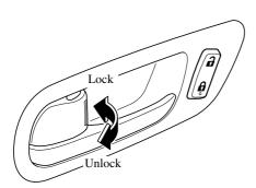
To lock any door with the door-lock knob from the outside, push the door-lock knob to the lock position and close the door. This does not operate the other door locks.
