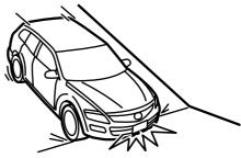
Your vehicle is equipped with low profile tires allowing class-leading performance and handling. As a result, the sidewall of the tires are very thin and the tires and wheels can be damaged if driven through potholes or on rough/uneven roads at excessive speeds. Use care and reduce speed when traveling on rough/uneven roads or through potholes.
