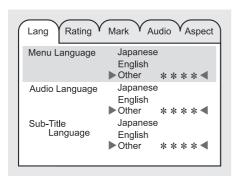
Move the cursor to the desired menu by operating the select button up/down or left/right. Press the ENTER button. The selected menu is highlighted to indicate that the menu is selected.
