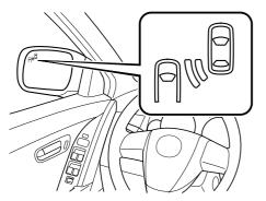
This warning light illuminates for a few seconds when the ignition switch is turned to the ON position.
