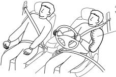
A side air bag will deploy only on the side the vehicle receives the force of the impact.
