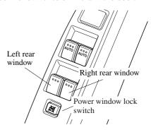
To open the power window to the desired position, hold down the switch. To close the power window to the desired position, pull up the switch.
