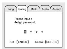
2. Press the ENTER button. If the password is confirmed, the password change mode is displayed.
