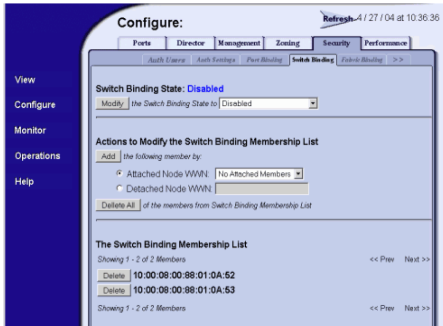
Figure 2-101 Configure Panel (Security Page with Switch Binding Tab)
