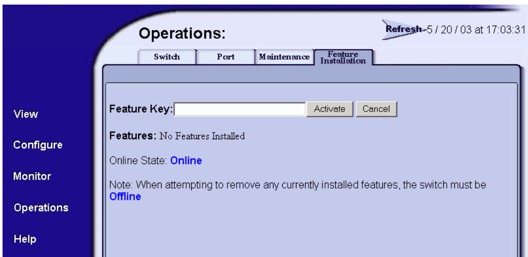
Figure 2-105 Operations Panel (Feature Installation Tab)
