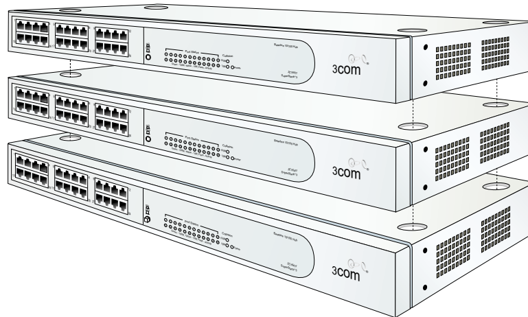
Figure 2-1 Stacked Ethernet Hubs
