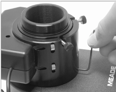
Fig. 62: Tighten the three microfocuser hex screws to a firm feel.
