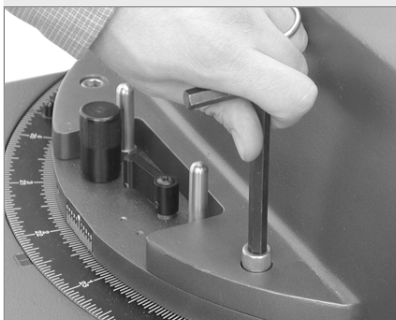
Fig. 51: Bolt the fork to the drive base.
