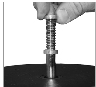
Fig. E, 2: Thread the first nut as far down as it will go. Then thread the second nut onto the first nut.
