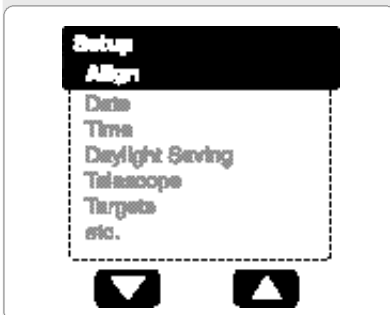
Fig. 15: Menu options display on the second line. Use the Scroll keys to move up or down through the list of options. Press ENTER to select the desired option.
