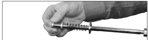
Fig. C: Remove 2 nuts and spring from threaded rod. Leave the washer on the rod.
