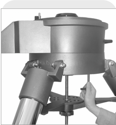
Fig. 50: Attach the drive base to the tripod.
