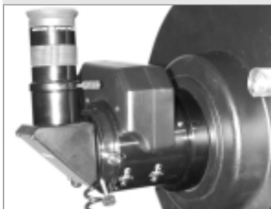
Fig. 9: Microfocuser and 1.25 diagonal prism with eyepiece completely assembled.
