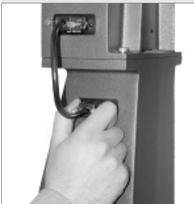
Fig. 54: Plug in the DB-9 connectors to provide power from the Dec. motor to the fork arms.
