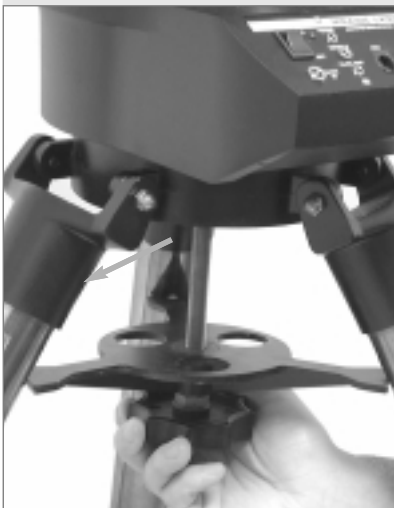
Fig. 4: Attaching the telescope to the tripod. Note the orientation of the spreader bar.
