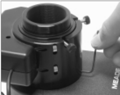
Fig. 60: Tighten the three microfocuser hex screws to a firm feel.
