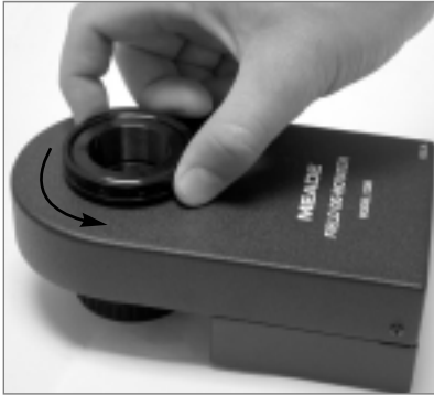
Fig. 58: Back off the adapter ring one full revolution.
