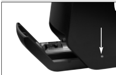
Fig. 55c: Location of one of the battery compartment screws. The other is located on the opposite end of the horizontal beam of the fork arms near the other battery compartment.
