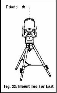
a. If the star drifts South (or down), the telescope's polar axis is pointing too far *East* (**Fig. 22**)
