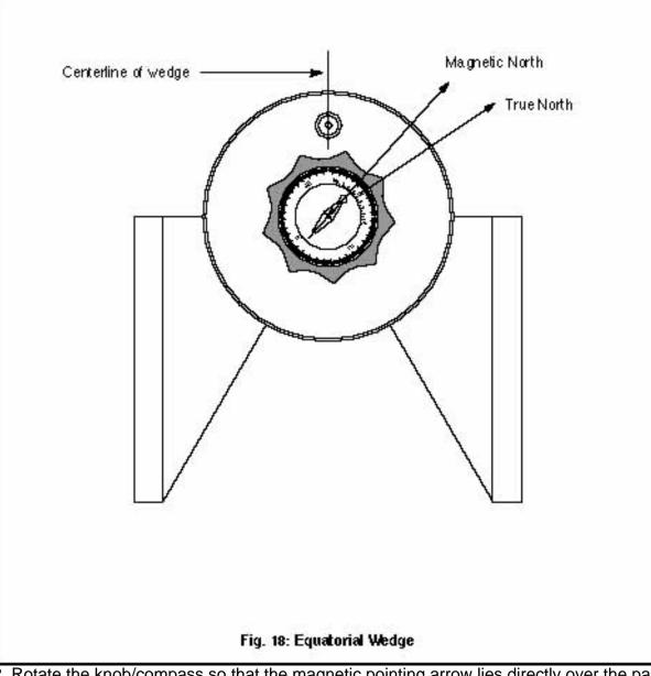
2. Rotate the knob/compass so that the magnetic pointing arrow lies directly over the painted black alignment arrow (painted on the bottom surface of the compass, **Fig. 18**). The "North" position on the direction scale (and the point on the knob/compass) now point directly north.
