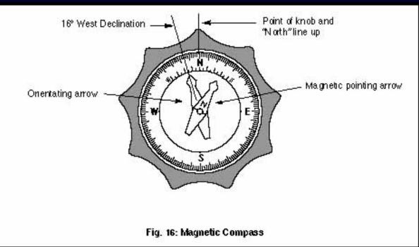
1. Snap the Magnetic Compass into the 3" diameter wedge attachment knob (after setting the Magnetic Declination as described above). Position the compass into the knob so that the 360 degree location on the direction scale (the "North" position) lines up with one of the nine points of the knobs. (**See Fig. 16.**) Press the compass firmly into the knob.
