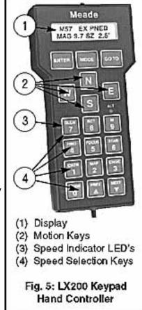
Hand Controller. Serious damage can occur to the internal gears of the motor assembly if the Declination Manual Slow-Motion Knob is turned even a slight amount by hand.
