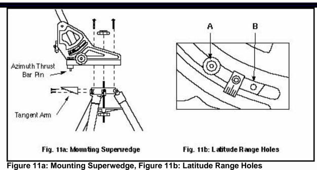
To assemble the Superwedge, follow this procedure (note that all required wedge hardware and manual knobs are shipped within the wedge carton):
