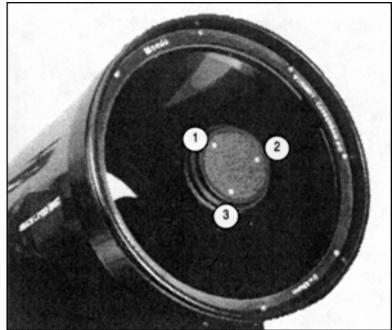
Fig. 26: Coillimation of the Optical System (1), (2), (3) Set screws for adjusting collimation.
