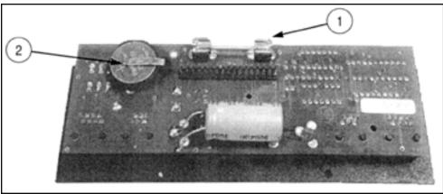
(1) Fuse (2) Battery Fig. 28: Reverse Side of Power Panel
