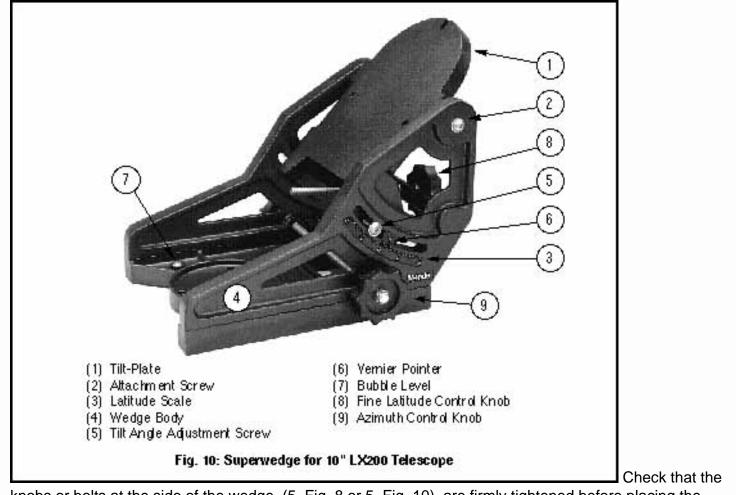
knobs or bolts at the side of the wedge, (5, Fig. 8 or 5, Fig. 10), are firmly tightened before placing the telescope onto the wedge.
