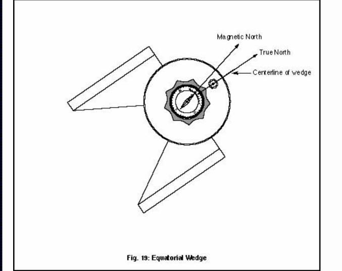
3. Rotate the Equatorial Wedge in azimuth (without moving the knob/compass) until the centerline of the wedge lines up with the point of the knob/compass (**Fig. 19**). The centerline of the Equatorial Wedge now falls directly on the true north line.
