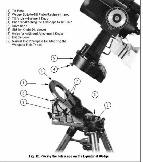
Thread one of these knobs (or screws, as appropriate) partially into the hole on the underside of the drive base, located at the curved-end of the drive base. See 4, Fig. 12. This knob or screw should be threaded in about 3 full turns, not fully threaded into the hole.
