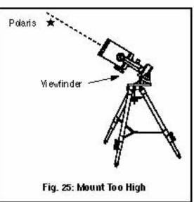
b. If the star drifts *North,* (or up) the telescope's polar axis is pointing too *high* (**Fig. 25**).
