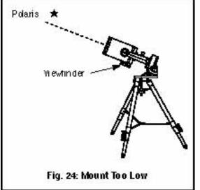
a. If the star drifts *South,* (or down) the telescope's polar axis is pointing too *low* (**Fig. 24**).
