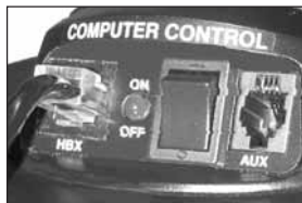
Fig. 12: Connect Audiostar to the HBX port.
