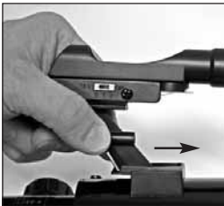
Fig. 8a: Slide viewfinder into slip-fit bracket.
