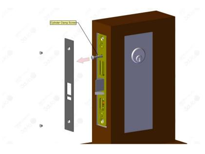
Using a key partially inserted, rotate the mortise cylinder counter-clockwise to remove it. Also remove any trim rings if they are used.
