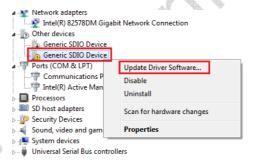
5. According user's Windows' OS to select and install test tool driver.
