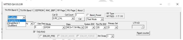
Users can check RF Type which should be shown MT7925B22M: 2 T 2 R to make sure the QA-Tool is working normally. There are two modes, BIN-file mode and E-fuse mode, supported by QA-tool. Section 2.2.2 & 2.2.3 provide details about respective mode.
