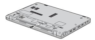
**6** Put the battery back in place. Turn the computer over and reconnect the cables.
