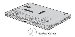
**6** Put the battery back in place. Turn the computer over and reconnect the cables.
