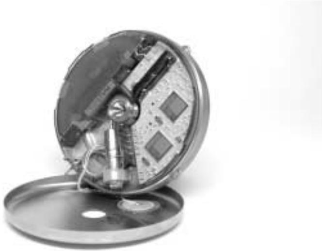
*Figure 2: Interior of the Implantable Insulin Pump*
