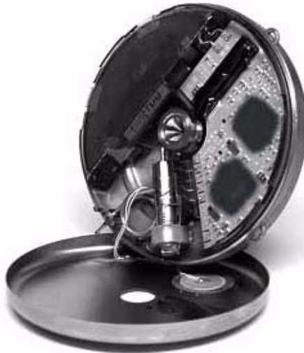
Figure 3: Interior of the Implantable Insulin Pump
