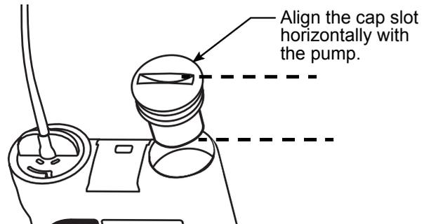
4. Turn the battery cap clockwise 4 half-turns so the slot is aligned horizontally with the pump as shown here:
